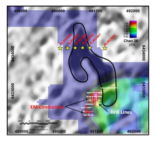
Figure 1. Plato Prospect: Existing RC holes and Proposed Drill Lines over FLEM Conductors
