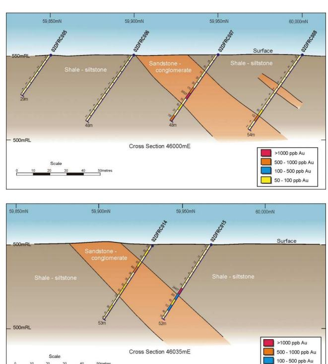
Figure 6: Drillhole Cross Section 46000E and 46035E, Doug's Find Prospect
