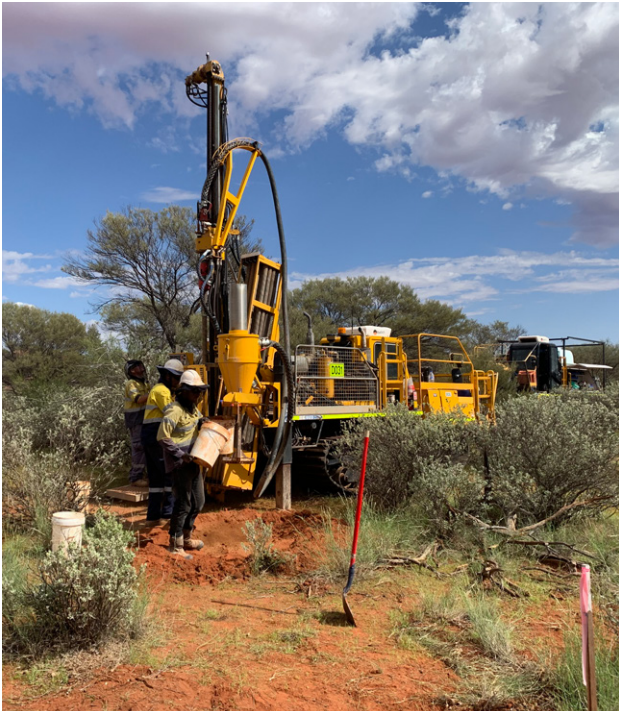
Figure 7. Aircore drilling by Evolution Mining Ltd along Big Bell Shear Zone
